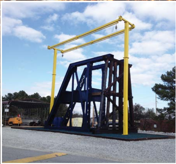
CSX recently designed and built a climbing structure for inspection training, helping to ensure safe bridge climbing techniques and high-quality inspections across the network.
